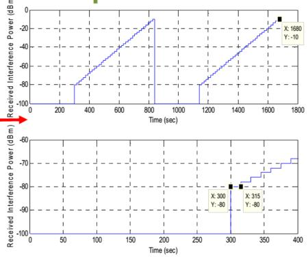
Nominal receive interference power profiles at GNSS antenna location for the (1520 to 1555 MHz) and (1645 to 1675 MHz) frequency ranges.
